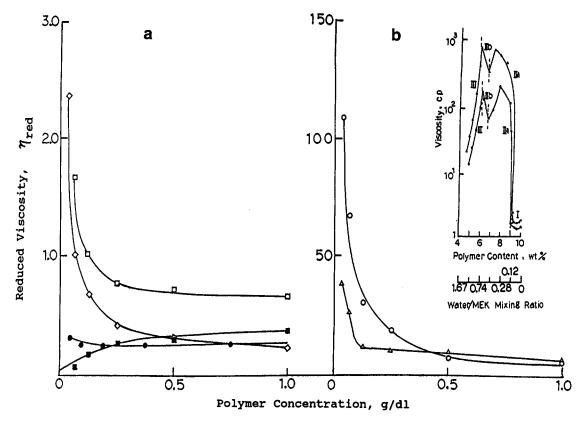
Figure 3 The reduced viscosity curves of sample M-0.7 in water/MEK with various mixing ratios (by weight): ( $\bigcirc$ ) 0.0, ( $\bigcirc$ ) 0.12, ( $\bigcirc$ ) 0.28, ( $\bigcirc$ ) 0.74, ( $\triangle$ ) 1.67, ( $\diamond$ ) 4.44. The insert is taken from ref. 20: (lower curve) M-0.7, (upper curve) M-1.0
