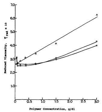
Figure 1 The reduced viscosity curves of the polymers with various ionic contents in MEK:  $(\triangle)$  M-0.0,  $(\Box)$  M-0.7,  $(\bigcirc)$  M-1.0
