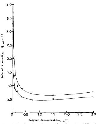
Figure 6 The reduced viscosity curves of emulsions: ( $\Box$ ) M-0.7, ( $\bigcirc$ ) M-1.0
