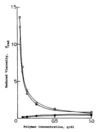
Figure 5 The reduced viscosity curves of the ionized samples in water/MEK and water/DMF with a mixing ratio of 0.12:  $(\blacksquare, \square)$  M-0.7,  $(\bullet, \bigcirc)$  M-1.0. The full symbols are for water/MEK and the open symbols are for water/DMF
