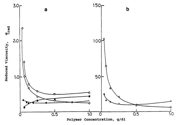
Figure 4 The reduced viscosity curves of sample M-1.0 in water/MEK with various mixing ratios (by weight): ( $\bigcirc$ ) 0.0, ( $\bigcirc$ ) 0.12, ( $\bigcirc$ ) 0.28, ( $\bigcirc$ ) 0.74, ( $\triangle$ ) 1.67, ( $\diamond$ ) 4.44
